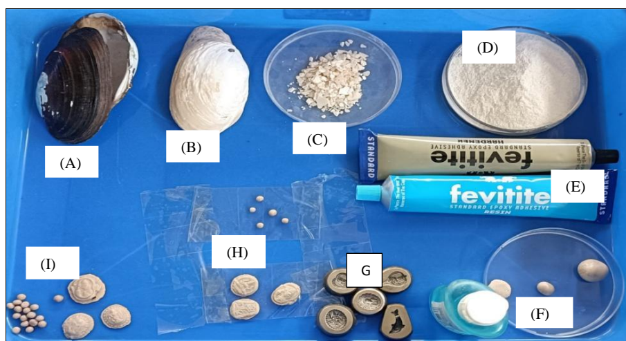
Fig 3: Procedural steps for preparation of bead or nucleus using the outer shell of mussels. Dead outer shells (A), cleaned shell (B), grinded shell (C), grounded powder (D), adhesive (E), dough prepared by outer shell (F), mold used for image bead preparation (G), and images for insertion in the mantle cavity (H and I)
