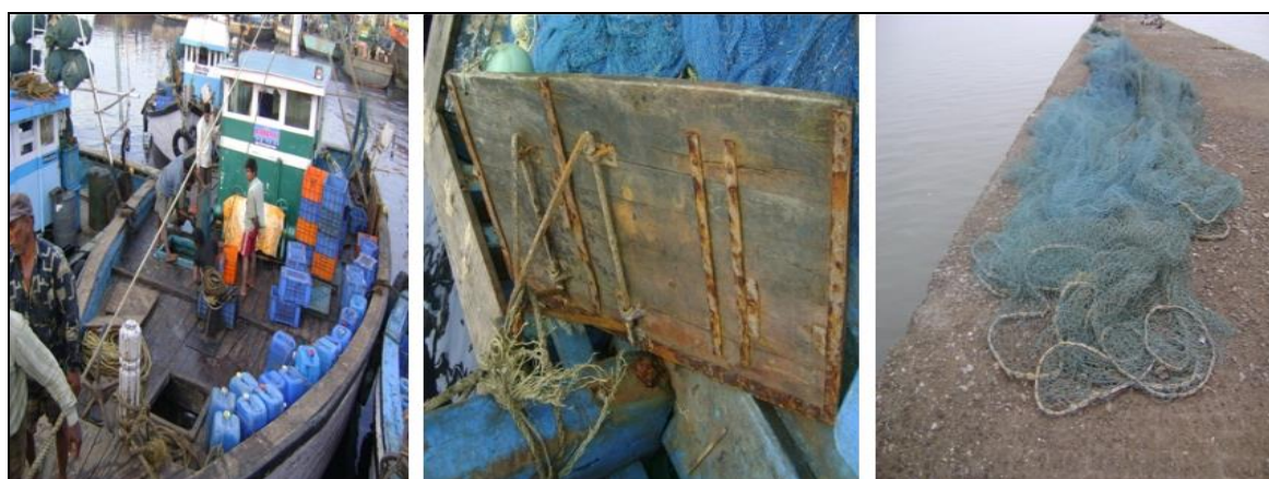
Fig 3: Trawl boat with otter board and trawl gear
