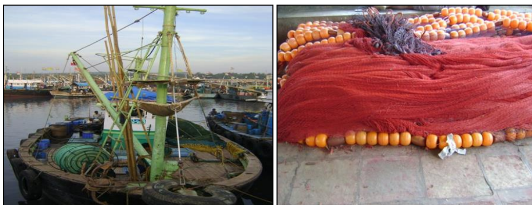
Fig 2: Purse-seine boat with purse-seine gear
