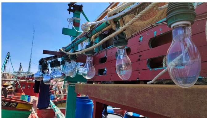
**Fig 10:** Metal halide lamp use in ASHBN vessel
