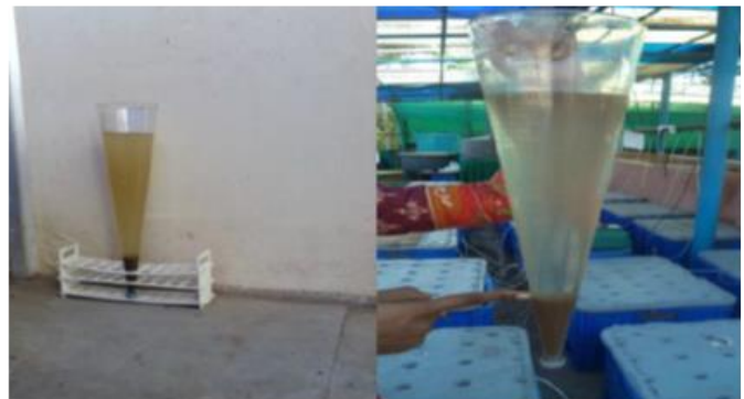
Fig 2: Observation of biofloc volume in imhoff cone
