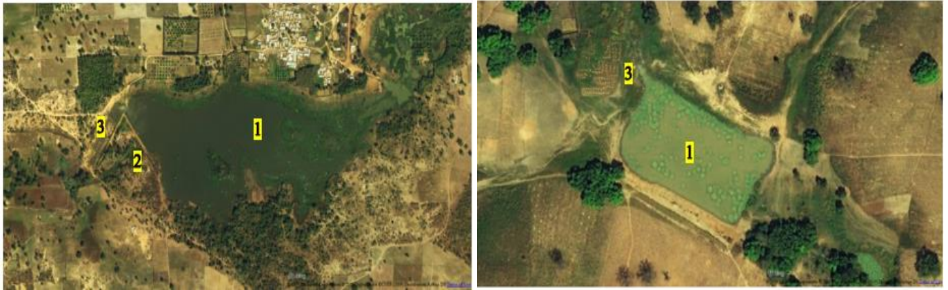
Fig 1: Differences between dam (A) and over dug pond (B) Sources: Google Earth & Bing Maps; Legend: 1 = bowl; 2 = dike and 3 = spillway (artificial channel in A or natural channel in B)
