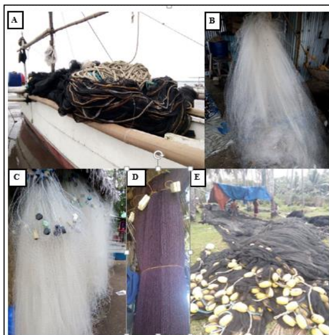
Fig 3: Fishing gears (nets) used in SIMBANA, Puerto Princesa City and Rasa Island, Narra, Palawan, Philippines: beach seine (A), bottom-set gill net (B), drift gill net - nylon (C), drift gill net - pamo (D), and ring net (E).
