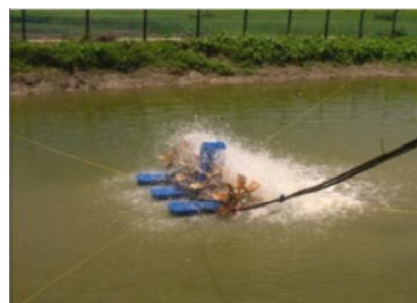
Fig 1b: Paddle wheel aeration in prawn rearing pond
