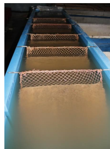
Fig 5: The incubation apparatus Tray Type
