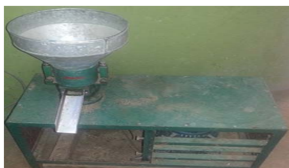
Plate 3.2: Powdery Feed Machine (Dry Pelletizer) (Machine A)
