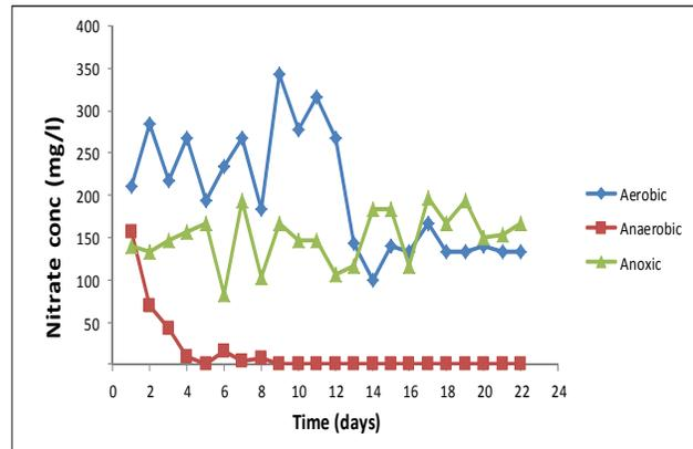
**Fig 7:** Average daily nitrate concentration in aerobic, anaerobic and anoxic reactors. No standard errors given.
