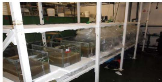
Fig 2: Diagram showing 9 reactors used for biofloc development. Open (aerobic reactors) covered (anaerobic and anoxic reactors).
