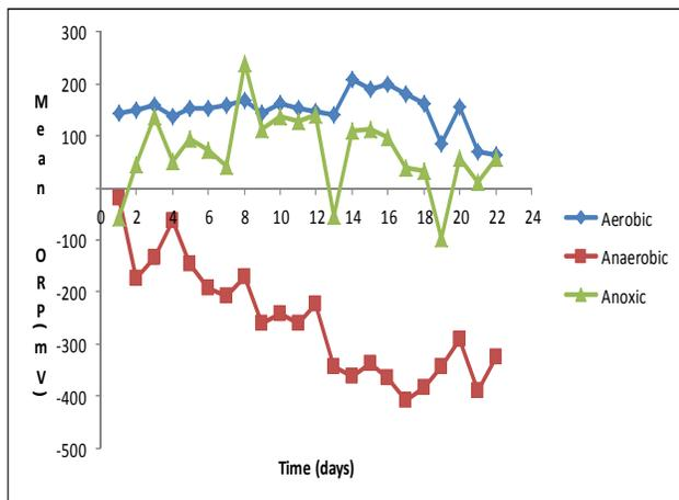
**Fig 6:** Average daily redox potential in aerobic, anaerobic and anoxic reactors. No standard errors given.
