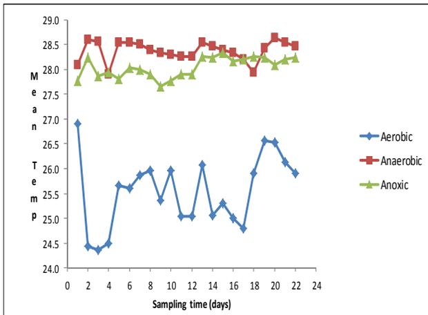
**Fig 5:** Average daily temperature in aerobic, anaerobic and anoxic reactors. No standard errors given.
