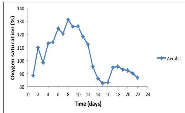
**Fig 8:** Average daily oxygen saturation in aerobic reactors. No standard errors given.
