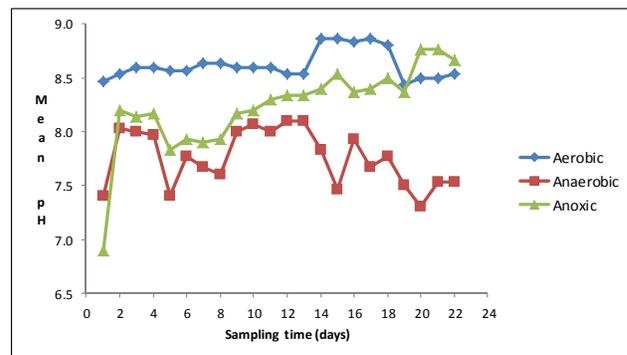
**Fig 4:** Average daily pH in aerobic, anaerobic and anoxic reactors. No standard errors given.
