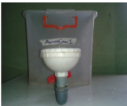
Plate 1: Upturned shower rose aeration column
