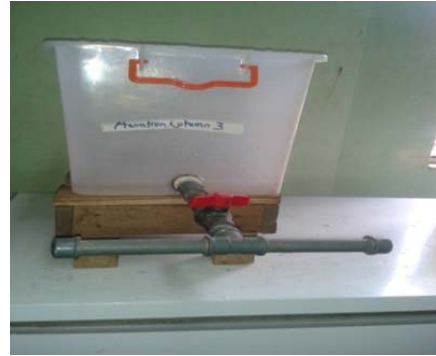
Plate 3: Perforated Pipe aeration column
