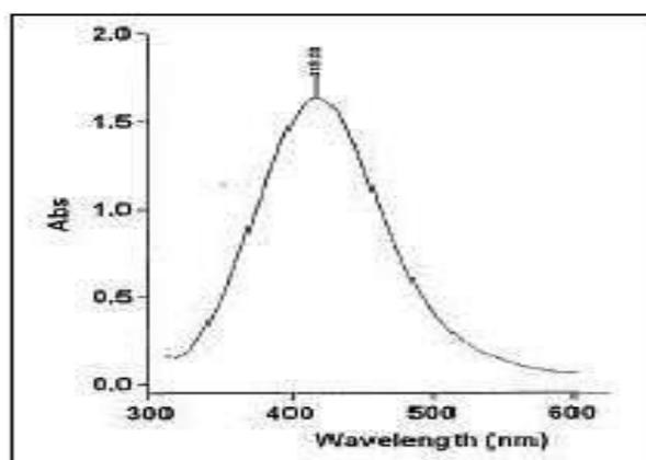
Fig 1: UV-Visible Spectrum of silver nanoparticles
