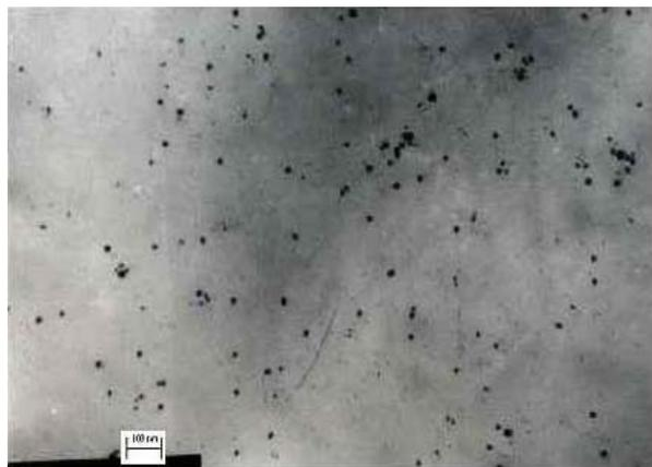
Fig 2: Transmission Electron Microscopic image of starch stabilized silver nanoparticles
