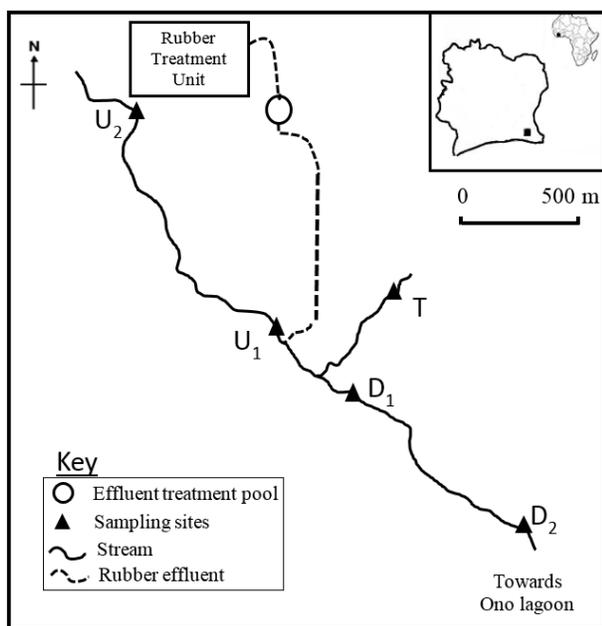
**Fig 1:** Sampling sites location. U1: Upstream site 1; U2: Upstream site 2; D1: Downstream site 1, D2: Downstream site 2; T: site on the tributary of river Wawa.
