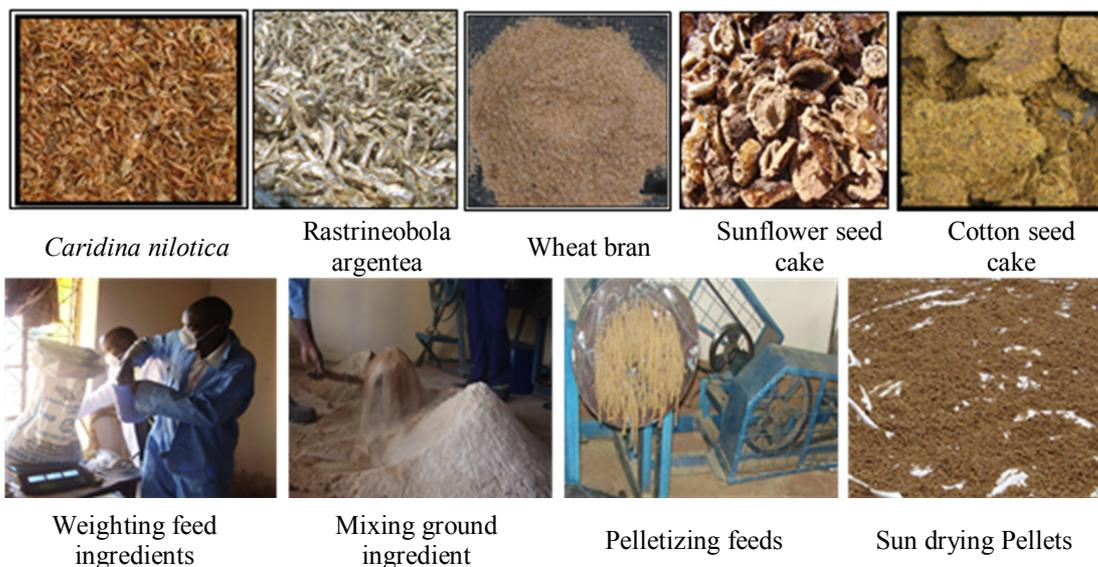
**Fig 6:** Photos showing some commonly used fish feed ingredients and feed formulation procedures in Kenyan fish feed industry <sup>18, 91</sup>
